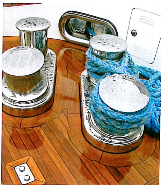
Mooring bitts in use: the deckhand can adjust the length of the line without having to remove it from the winch.
